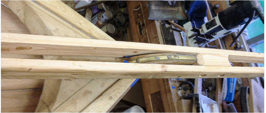
Rudder hanging copied from the Shetland double ender
