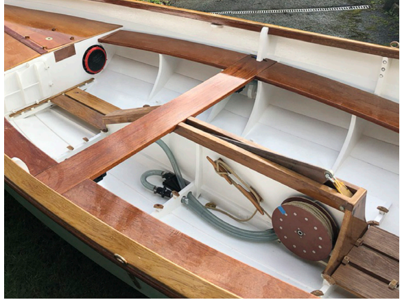
Two manual bilge pumps installed crossed over
