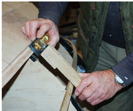
A block plane with wood spacer bolted to it being used to plane the bevel
