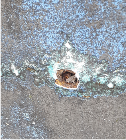
Bubbling paint concealed a hole in the hull
