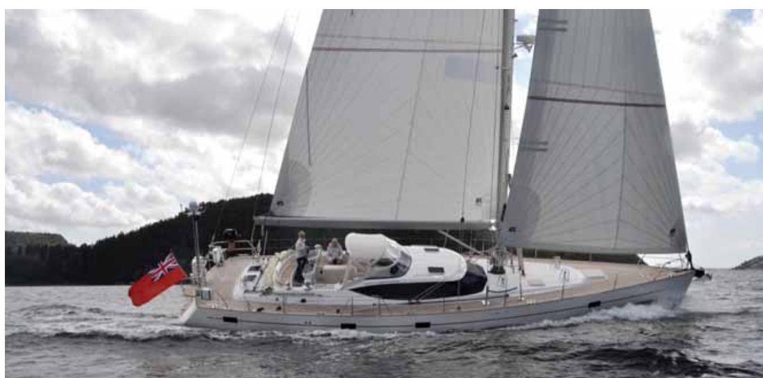
The twin jibs flying in tandem, with their own colour-coded sheets, fairleads and winches
