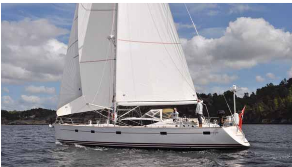
The mainsail directs its wind around the mast into the weather jib, which redirects its total accumulation into its leeward twin
