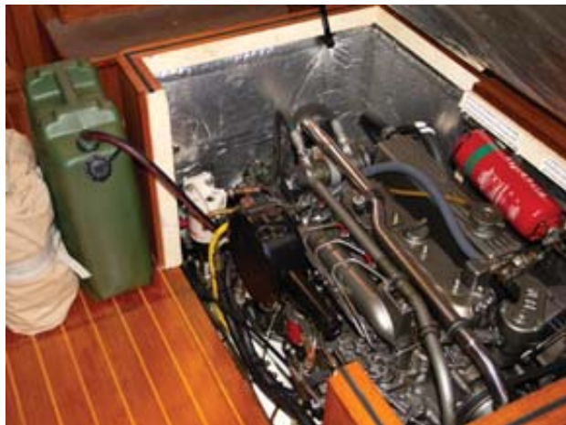
The jury-rigged fuel system. The jerry can was subsequently lashed in place to stabilise it against a slight rolling sea
