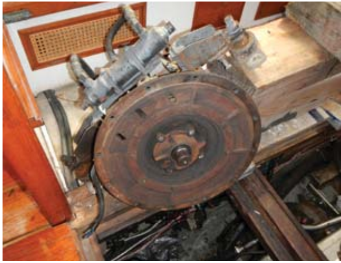
The flexible coupling disassembled from the gearbox
