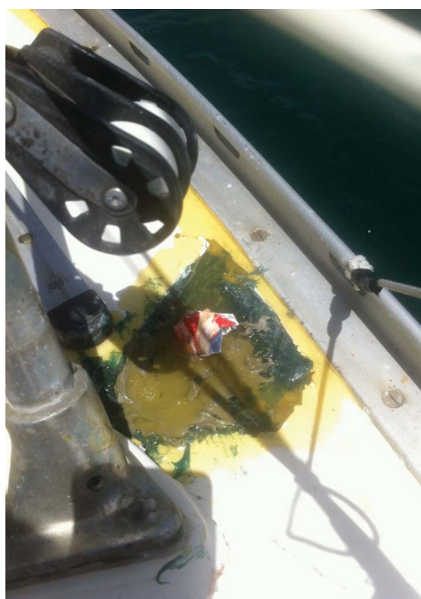
The hole in the deck, finally fixed with resin and Plastic Padding
