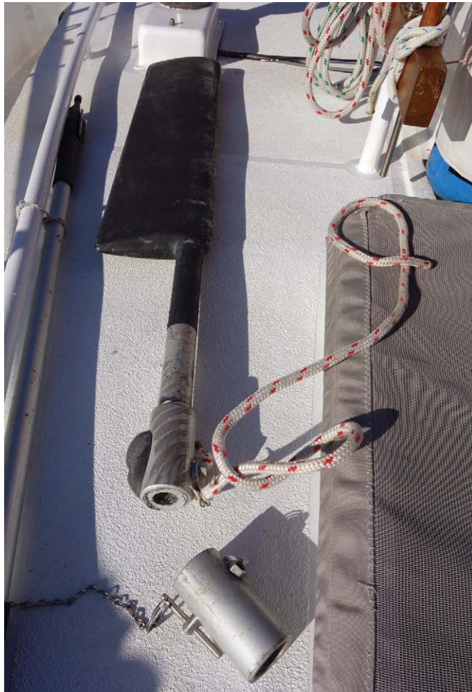
The sheared Aries paddle on Ironhorse's coachroof, showing both halves of the broken sleeve
