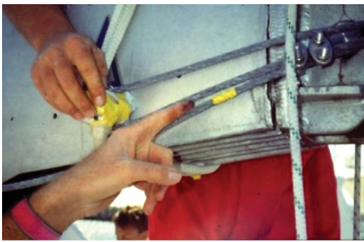
The crack around the forward end of the boom
