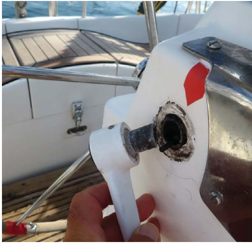
The throttle lever wrenched from the steering column
