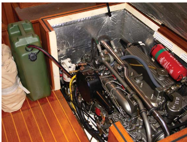
The jury-rigged fuel system. The jerry can was subsequently lashed in place to stabilise it against a slight rolling sea
