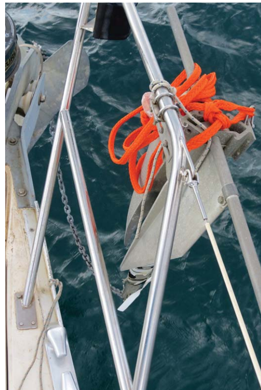
The Fortress still in its bracket but with the securing lines freed and awaiting deployment. Note the chain shackled to the eye of the Delta
