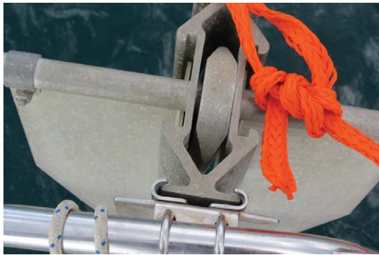
The Fortress nestled in its bracket on the rail with a polypropylene rope attached. The bracket is adjustable for wider 'fluke heads' (for want of a better term)
