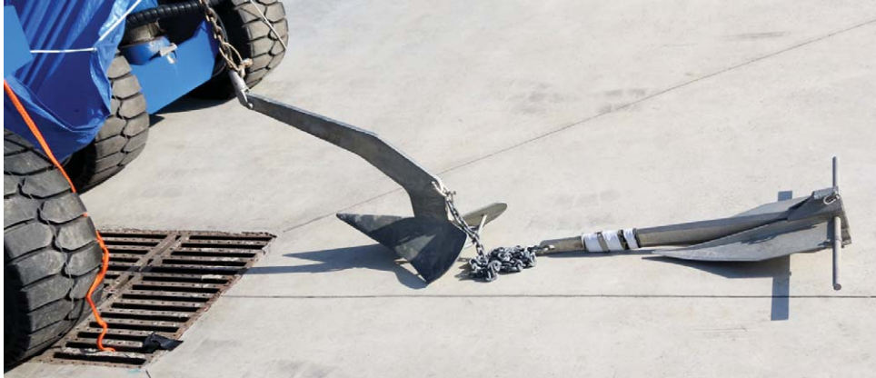
The Fortress deployed on the 'seabed', with the Delta ready to be set in reserve. Note the shackle on the former's crown, to which a tripping line would be attached
