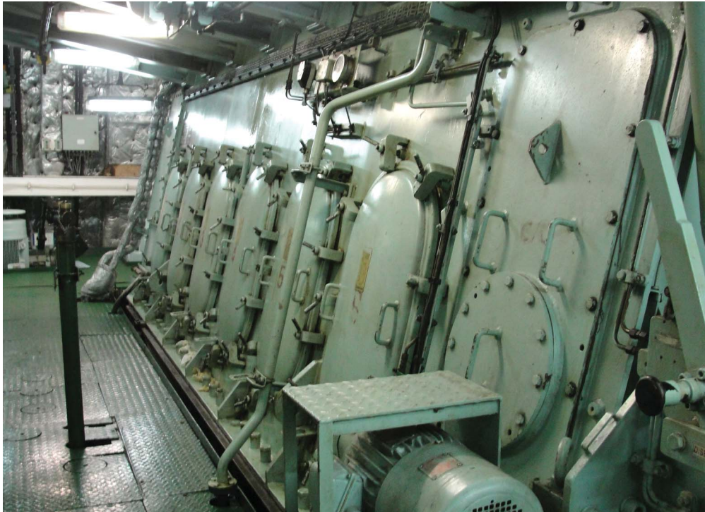
The reverse side of the engine with walk-in inspection hatches
