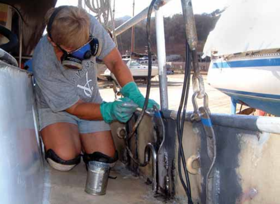
Applying 'Rust Rebel' to the damaged paintwork behind the newly-welded chainplates
